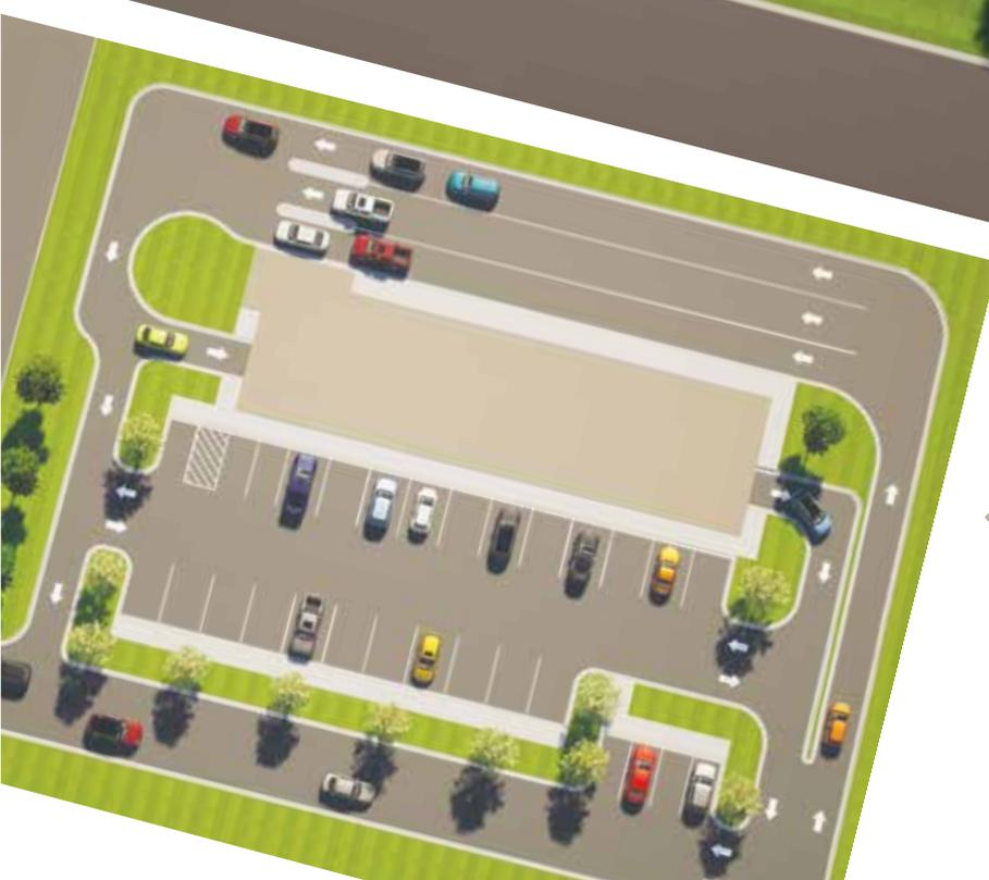
◀ A CONVENTIONAL SHOTGUN STYLE LAYOUT WITH RIGHT ANGLE VACUUM PARKING. THIS IS A GENEROUS SITE AND HAS ROOM TO EXPAND THE LAYOUT TO THE VERY EDGES TAKING INTO ACCOUNT ALL THE USEABLE SPACE.
