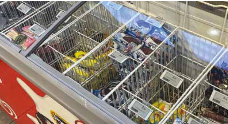
Electronic shelf labels in a frozen foods section, displaying pricing on refrigerated products.
